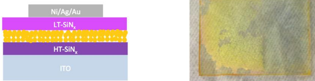
Fig. 1 (left) Schematic representation of the cross-section of the fabricated device. A layer of QDs is sandwiched between two layers of SiN x with a top and bottom electrical contact. (right) Picture of cracked SiN x layer when using a top low temperature and low frequency deposition on QD layer.
